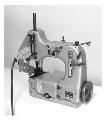
This kit eliminates awkward foot pedal action and simplifies guiding the bag into the sewing head, effectively deskilling the bag closing operation. It also insures consistent, reliable closures and contributes to increased production.
