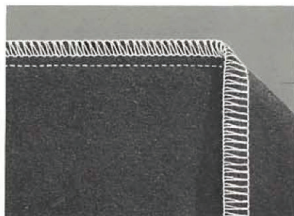
Sample of overseaming produced with Style 39500 QW. Notice similarity in appearance to "Safety-Stitch".
