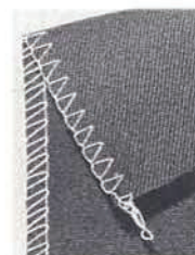
Style 39500 QJ produces two-thread stitch, Type 503
