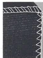
Style 39500 QL produces three-thread stitch, Type 505
