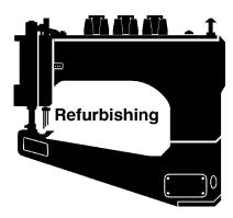
Union Special has recently incorporated sewing machine refurbishing into its customer support. Union Special machines that are sent in are completely disassembled, castings sanded and repainted, bushing tested and replaced as needed, parts checked and repaired or replaced as needed and the machine is reassembled, adjusted to Union Special spec's, sewn-off and repacked in a new box for returned to the customer. (Currently only 35800, 36200, 39500 & 56000 styles are being refurbished.)
